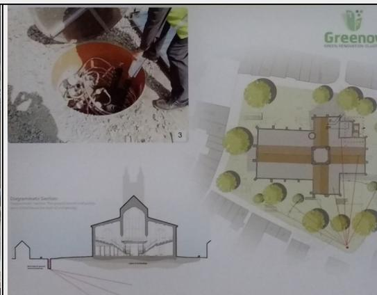
**3** This detail from a public information panel shows the plan and elevation views of the boreholes. All of the pipework is accessed from one master manhole, pictured top left.
