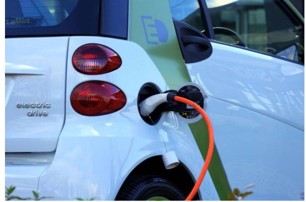
Charging points allow electric cars to be plugged in to recharge their batteries. This can be a quick pit stop using a rapid charger, where the driver is only stopped for 20-30 minutes, or it can be a more gradual charge over a few hours, whilst the driver is at work, school, or church.
