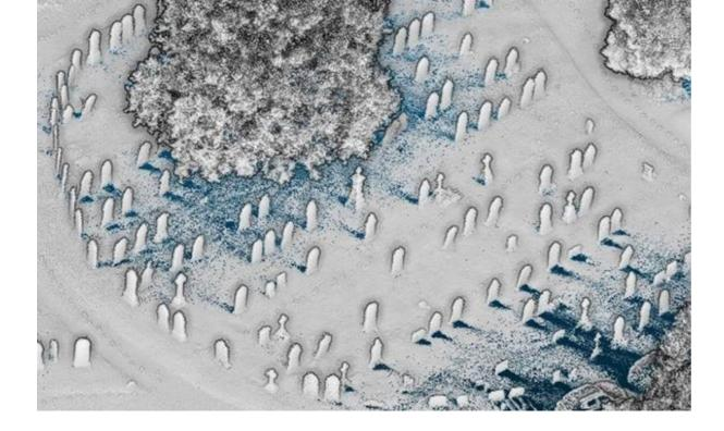
Use of the latest surveying equipment and bespoke software built by Atlantic Geomatics has made the national-scale survey a possibility for the first time. Operatives will aim to survey around nine or ten sites a day using back-pack mounted laser scanning equipment, GPS and cameras. Taking tens of thousands measurements every second the surveyors will then process the data to create accurate maps of each churchyard.
