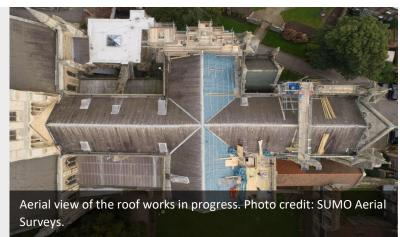
masonry below, and for repairs and weather proofing to weak, buckled and leaking stained glass and clear glazing. Falling masonry presented a danger to the public and would have required closing the north door, the main entrance of the cathedral for visitors and the only level access point.
