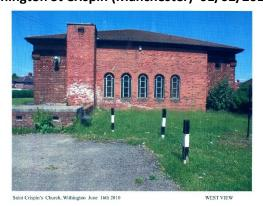
Large building with serious inherent and deteriorating structural faults; in very poor state of repair and costs beyond means of parish. Congregation (around 30) found building too large for its needs and currently worshipped in church hall. 1981 survey estimated costs in excess of £371k (included foundation and wall tie failure). Adjacent church hall to be refurbished into new place of worship.
